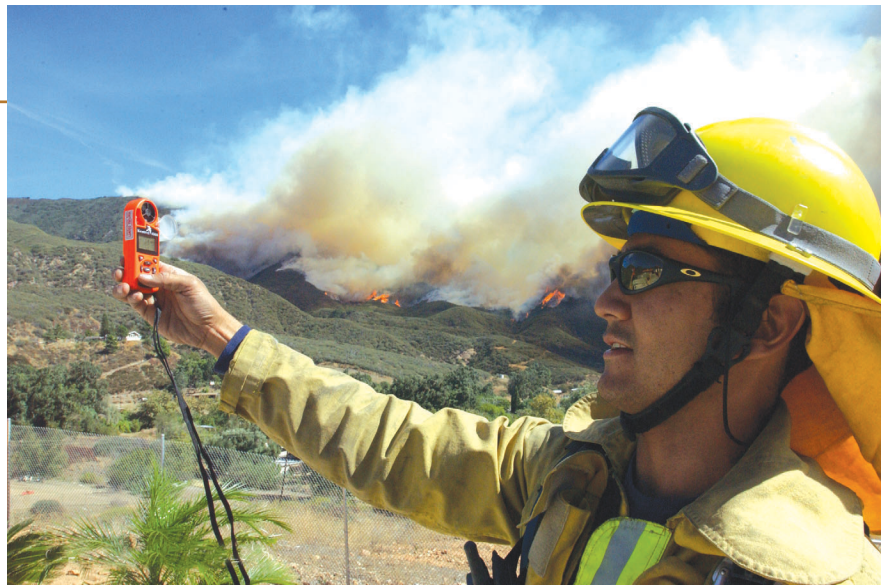
A firefighter checks the wind conditions by using a Kestrel weather instrument.
